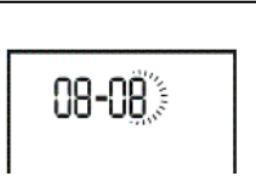
7. The day flashes on the display. Use the START button to select the current day and confirm using the ON/OFF button
