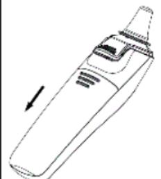
3. Insert two new 1.5 V AAA batteries. Make sure that the batteries are inserted the right way round. Close the battery compartment.
