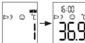
4. If you would like to proceed with a measurement, press the START button. Press and hold the ON/OFF button
